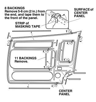
5. Attach a strip of masking tape to the end of each shaded backing. Peel back 5-6 cm (2 in.) of the backings and fold them over as shown. Temporarily attach the strips of masking tape to the front surface of the center panel. Remove all remaining backings from the center panel.
