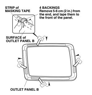
10. Position outlet panels A and B on the existing outlet panels. While holding pressure on the outlet panels, carefully remove the backings from the outlet panels. Hold outlet panels A and B firmly against the existing outlet panels with the palm of your hand, particularly at the edges.
