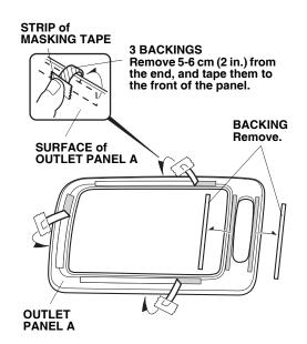
8. Attach the strip of masking tape to the end of each shaded backing. Peel back 5-6 cm (2 in.) of the backings and fold them over as shown. Temporarily attach the strips of masking tape to the front surface of the outlet panel A. Remove all remaining backings from the outlet panel A.
