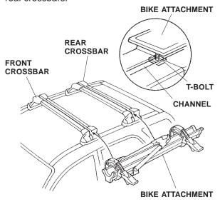
7. Turn and adjust the mounting lever to lock the bike attachment to the roof rack. Check for firm pressure while you push down on the mounting lever to lock it into place.
