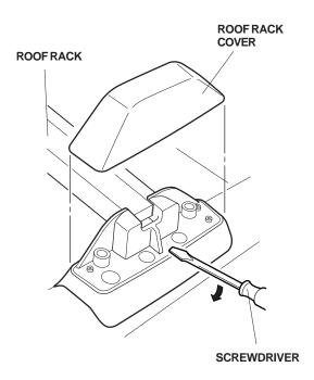
Remove the rubber moldings from the front and rear roof rack crossbars. Retain the rubber moldings to reinstall if the bike attachment is removed.
