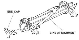
Turn and loosen the mounting levers on the bike attachment.
