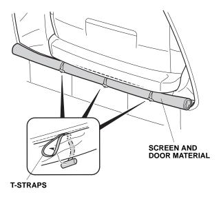
8. Stretch the bottom elastic strap across the rear face of the bumper. Make sure the tent material is tight against the rear face of the bumper, with the exhaust pipe outside the tent. Go outside of the tent, and make sure the exhaust pipe is outside.
