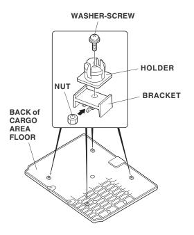
3. Unfold the table legs, and place the cargo area floor holders into the square holes of the table legs.
