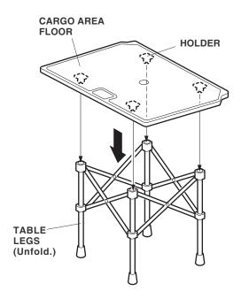
4. Confirm that the table legs and the holders have been installed securely.
