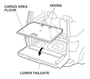
Turn the cargo area floor over, and slide one nut into each of the four brackets as shown. Install the four holders onto the brackets, and secure each holder with a washer-screw.
