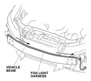
33. Secure the clip to the vehicle frame as shown.
