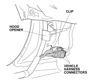
43. Remove the vehicle harness connector from the vehicle harness 13-pin connector.
