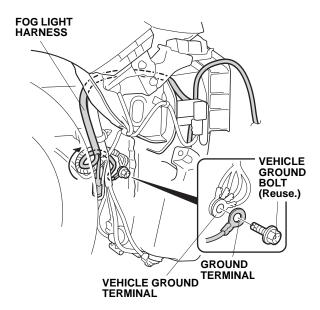
28. Attach the fog light harness ground terminal to the vehicle ground terminal, and reinstall the vehicle ground bolt.
