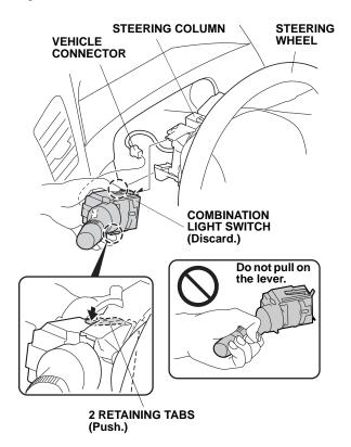
59. Push the two retaining tabs and slide the combination light switch out of the steering column. Do not pull on the lever when removing the switch.
