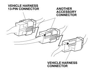
44. Remove the clip from the vehicle harness 13-pin connector, and install clip B on the 13-pin connector.
