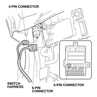
Using two wire ties, secure the switch harness to the vehicle harness.
