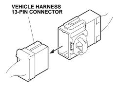
46. Release the retainer on the vehicle harness 13-pin connector. Insert the switch harness terminal into the 13-pin connector as shown.
