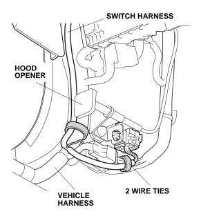
57. Using two wire ties, secure the switch harness to the vehicle harness.
