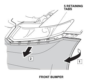
With the help of an assistant, remove the front bumper (two hex bolts and two clips). Place the front bumper on a blanket to prevent damage.
