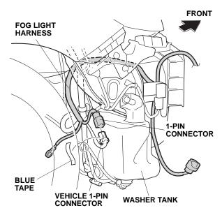
25. Plug the fog light harness 1-pin connector into the vehicle 1-pin connector as shown.
