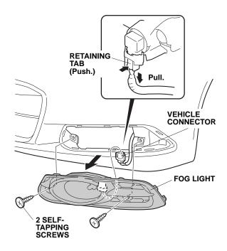
2. Remove the bulb from the fog light as shown.
