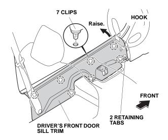
4. Pull away the door opening seal, and remove the driver's kick panel (two clips).
