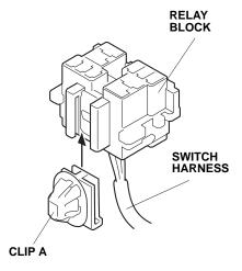
51. Install the relay on the switch harness relay block.
