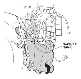
30. Using four wire ties, secure the fog light harness to the vehicle harness. Do not secure the fog light harness to the washer tube.
