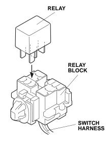
52. Secure the switch harness relay block to the relay bracket.
