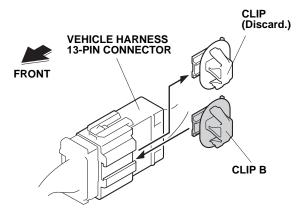
45. Unplug the vehicle harness 13-pin connector.
