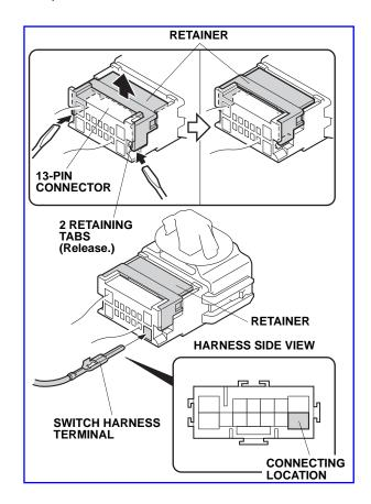
47. Reattach the other vehicle harness connectors to the vehicle harness 13-pin connector. Clip the connectors to the vehicle panel.
