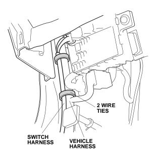
58. Unplug the vehicle connector from the combination light switch.
