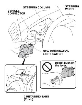
61. Plug the vehicle connector into the new combination light switch.
