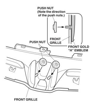
Reinstall the front grille. Install the two middle clips first, then the outer clips. Check that the clips are installed securely.
