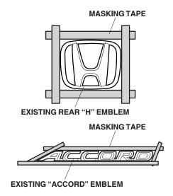
8. Remove the "H" and "ACCORD" emblems from the body by moving the string back and forth, and working it between the emblems and body.
