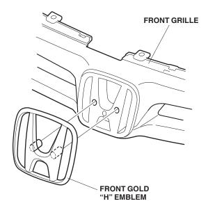
Slide the push nuts onto the pins. Note the direction of the push nuts.
