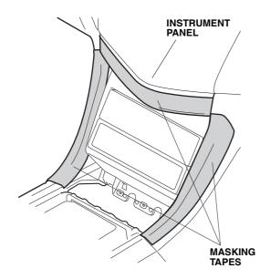
24. Remove the player panel (two self-tapping screws and two clips).
