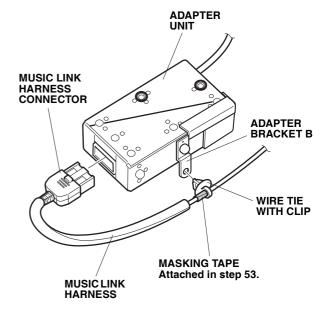
53. Install the adapter unit to adapter bracket A with two 5 x 8 mm bolts, two 5 mm plain washers, and match the marks made in steps 42, 45, and 47.
