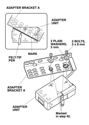
43. Using a felt-tip pen, mark the installation position of the adapter bracket A on the adapter unit.
