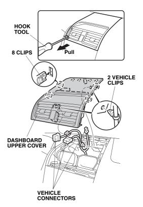
29. Remove the center panel (three self-tapping screws, two bolts, five clips and disconnect the vehicle connectors).
