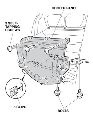
30. Remove the passenger's under cover (three clips and three pins).
