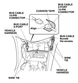
68. Secure the adapter unit harness and the Music Link harness to the vehicle harness with two wire ties.
