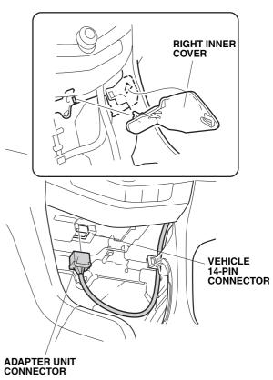
63. Bundle the excess adapter unit harness so that it does not come into contact with the right inner cover. Secure the adapter unit harness to the vehicle harness with two wire ties. Tighten two wire ties loosely, move a bundle of the adapter unit harness toward the front and then tighten the two wire ties securely. Go to step 82.
