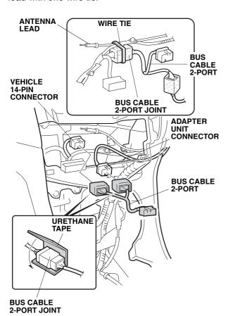
76. Connect the bus cable 2-port and antenna lead to the navigation unit.
