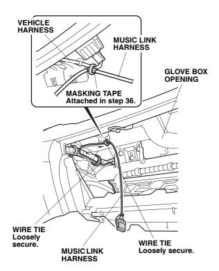
59. Bundle the excess Music Link harness and secure it to the vehicle harness with two wire ties loosely secured in step 60.
