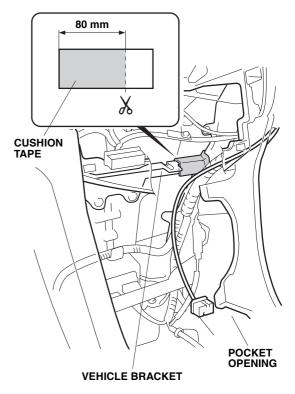
72. Align the vehicle 20-pin connector of the adapter unit at the center panel opening and secure the harness of the adapter unit to the vehicle harness with three wire ties as shown.
