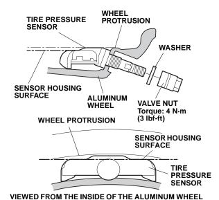
Install the tire pressure sensor and the washer to the aluminum wheel, and loosely install the valve nut. Make sure the pressure sensor is resting on the wheel.
