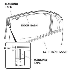
10. Using isopropyl alcohol on a clean shop towel, clean the area where the visor will attach.
