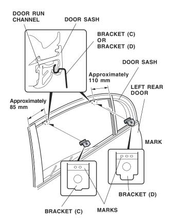
Install one bracket (C) and one bracket (D) on the door sash at the measurements shown. Verify the shape and the identification mark stamped on each bracket. Be sure to use the correct bracket at the proper location. 3. Position the left rear door visor on the door sash.
