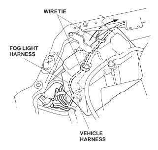
18. Attach two wire ties with clip to the fog light harness at the green-taped positions, then push the clip into the holes in the harness bracket.
