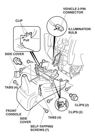
33. On M/T vehicle only, remove the two clips and seven self-tapping screws, and pull the front console out toward you to release four clips. Unplug the 2-pin connector from the accessory socket, and remove the front console. 34. Route the switch harness 5-pin connector into the instrument panel opening.
