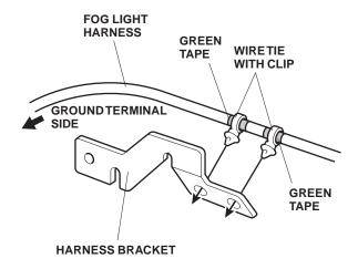
19. Remove two bolts that secure the air intake. Insert the harness bracket between the air intake and the bulkhead, then secure it with the two bolts. Secure the fog light harness to the vehicle harness with two wire ties.
