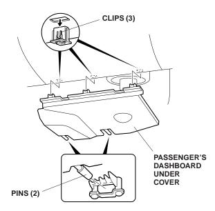
27. Open the dashboard pocket lid. Remove the lid by releasing the two retaining clips and two retaining tabs, then remove the dashboard pocket (one selftapping screw, then pull out to release the one clip and three retaining tabs). Unplug the vehicle connector.
