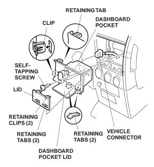
28. Remove two self-tapping screws that fasten the heater A/C control panel to the dashboard. Pull the heater A/C control panel out toward you to release the four clips. Unplug the vehicle connector, and remove the heater A/C control panel.
