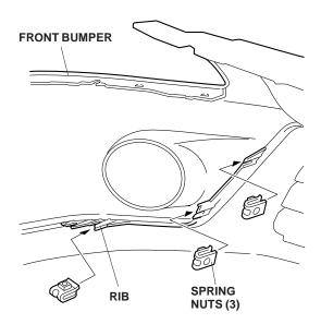
9. Fit the pin from the left fog light into the recess in the front bumper. Position the left fog light over the three holes in the spring nuts, and install the three washer-bolts.
