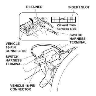
46. Lock the retainer, and plug the vehicle connector back into the combination switch.
