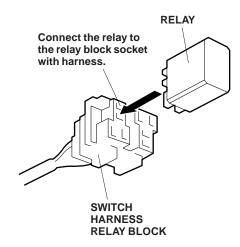
36. Slide the switch harness relay block onto the appropriate bracket, as shown.
