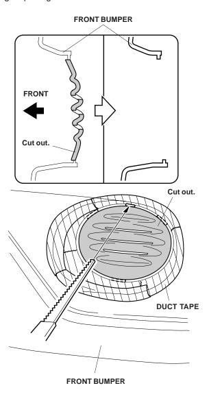
6. Using a hacksaw blade, slowly and carefully cut out the fog light opening. Be sure to cut the opening as round as possible, and do not damage the bumper. Remove any burrs from the edges of the fog light opening with a file.
