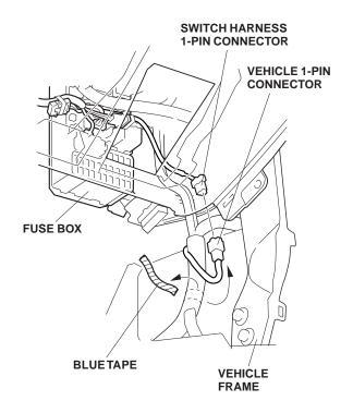
43. Route the switch harness terminal along the vehicle harness above the steering column.
