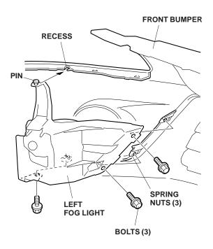
10. Repeat steps 5 through 9 to install the fog light on the right side of the vehicle.
