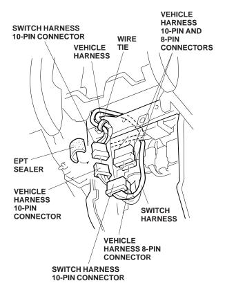
51. Secure the switch harness to the vehicle harness with one wire tie in the area shown.
