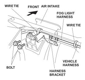
20. Route the fog light harness along the vehicle harness through the hole in the body panel. Secure the fog light harness to the vehicle harness, and to the bulkhead upper frame with the six wire ties in the areas shown.
