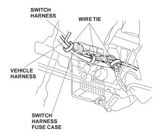
53. On vehicles with the vehicle 1-pin connector on the rear of the vehicle frame: Secure the switch harness to the vehicle harness with four wire ties. Secure the switch harness fuse case on the upper side, so the fuses in the fuse box can be accessed, and so that the vehicle bracket edge does not cut into the switch harness.
