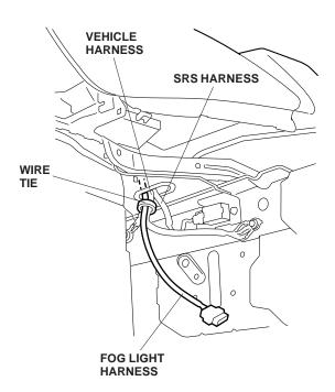
22. With an assistant holding the bumper, connect the two fog light harness 2-pin connectors to the left and right fog lights, then reinstall the front bumper. Do not fasten the inner fender (four clips and two self-tapping screws) to the front bumper until after the fot light aiming adjustment.
