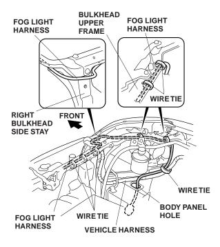
21. Secure the fog light harness to the vehicle ground harness with one wire tie. Do not secure the fog light harness to the SRS harness.
