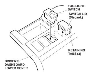
56. Install the fog light switch in the driver's dashboard lower cover.
