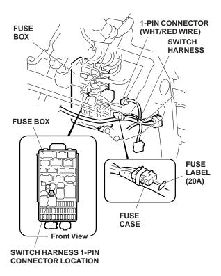
39. Connect the switch harness 1-pin connector (WHT/RED wire) to the fuse box.
