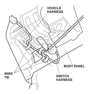
38. Attach the fuse label (20A) to the switch harness fuse case.
