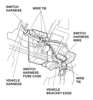
54. Along the steering column, secure the switch harness to the vehicle harness with two wire ties.
