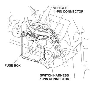
42. On vehicles with a vehicle 1-pin connector on the rear of the vehicle frame: Locate the 1-pin connector blue-taped to the vehicle harness, remove the blue tape, and free the connector. Connect the switch harness 1-pin connector to the vehicle 1-pin connector.
