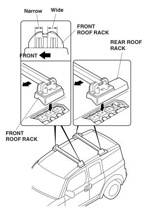
6. If the ends of the right and left roof racks are not aligned, adjust them by loosening the crossbar socket bolts, and moving the stays in or out as necessary.
