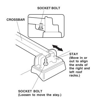
7. Install the roof racks with 12 socket bolts and 12 washers. Do not tighten.
