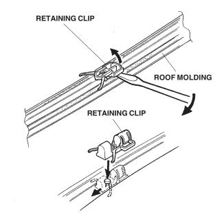
4. If any of the six center retaining clips remained on the roof, remove them from the stud bolts using long nose pliers.
