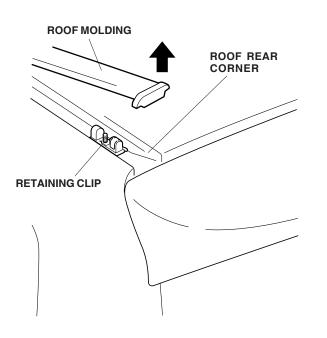
3. If the front or rear retaining clips remained on the roof molding, remove them from the roof molding, and reinstall them in their original positions on the vehicle. Remove the remaining clips and set them aside; they will not be reused.
