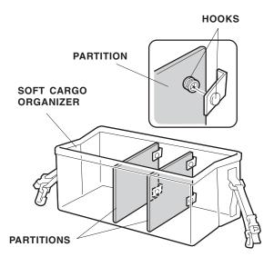
Place the organizer in the cargo area of the vehicle, and attach the outer hooks of the organizer to the vehicle tie-down hooks.
