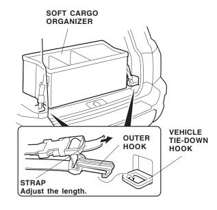
Adjust the length of the strap as needed to secure the organizer to the tie-down hooks.
