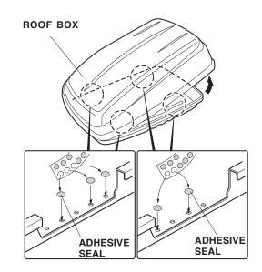
2. Using isopropyl alcohol on a shop towel, clean four brackets B where the small pads will attach. Remove the backings from the small pads and attach them to the brackets B.
