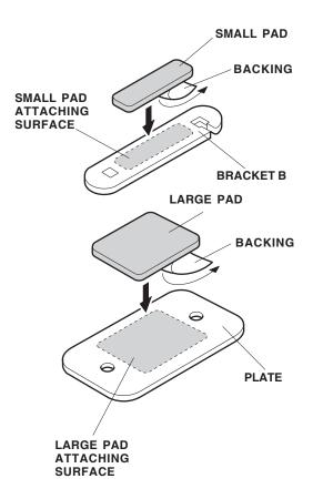
3. Using isopropyl alcohol on a shop towel, clean four plates where the large pads will attach. Remove the backing from the large pads and attach them to the plates.
