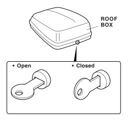
**Locking**: Press down on the lid. There should be an audible click. Be sure the lid is latched by attempting to lift the lid. Turn the key clockwise to lock the roof box. Remove the key while not in use. Be sure the straps are not outside of the roof box.
