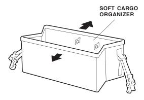
2. Attach the two partitions to the soft cargo organizer by connecting the inner hooks.
