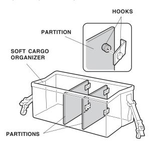
3. Place the organizer in the cargo area of the vehicle, and attach the outer hooks of the organizer to the vehicle tie-down hooks.
