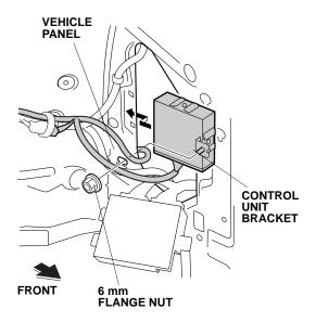
36. Secure the backup sensor harness to the vehicle harness with one wire tie.
