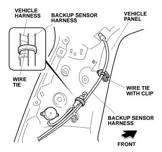
43. Secure the backup sensor 8-pin connector to the vehicle panel.
