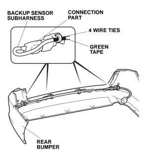
62. Using isopropyl alcohol on a shop towel, throughly clean the area where the harness tape will attach. Secure the backup sensor subharness to the rear bumper with three harness tapes.
