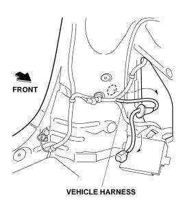
18. Bundle the vehicle harness as shown and secure it to the vehicle harness with one wire tie.
