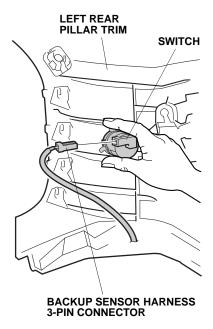
51. For the left rear pillar trim, insert the clip matching the upper tab and install the trim. At the time of installation, take care that the switch does not come into contact with the left rear pillar trim.
