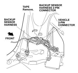
26. Remove the blue tape from the backup sensor harness. Plug the backup sensor harness 2-pin connector to the vehicle harness 2-pin connector.
