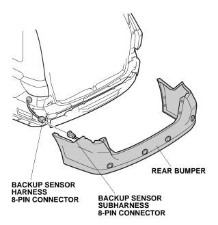
64. Install the rear bumper back onto the vehicle.
