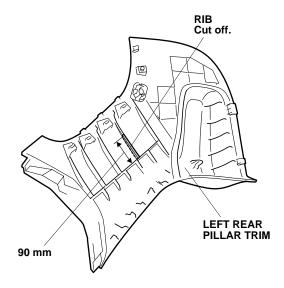
45. On the inside of the left rear pillar trim, measure from the inside of the ribs, and mark the pillar trim at the measurements shown. While wearing eye protection, drill a 3 mm hole at the marked position. Then drill with a 26 mm hole saw.
