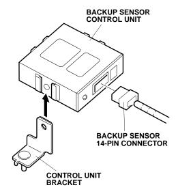
35. Attach the backup sensor control unit to the vehicle panel and secure the control unit bracket with 6 mm flange nut.
