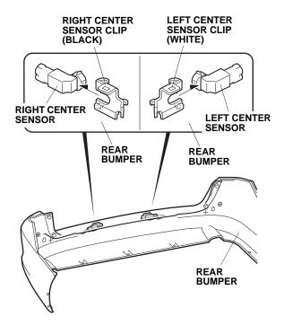
58. From the outside of the rear bumper, insert the two corner sensors into the holes as shown. Make sure that the sensor is inserted into the instructed hole.
