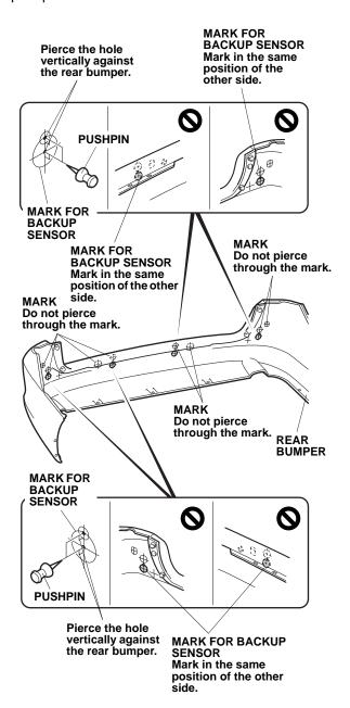
54. While wearing an eye protection, drill 3 mm hole at the four pierced marks on the corner of the rear bumper from the outside. Widen the two lower holes with 24 mm hole saw as shown. Remove any burrs.
