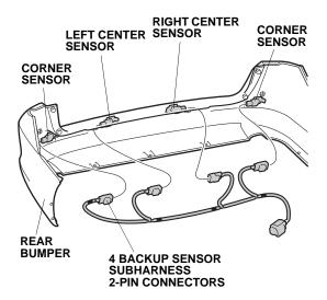
61. Secure the backup sensor subharness to the sensor clip at the green tape with four wire ties as shown.
