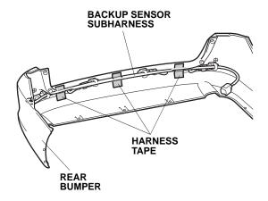
63. Bring the rear bumper to the vehicle and plug the backup sensor subharness 8-pin connector to the backup sensor harness 8-pin connector.
