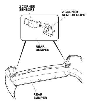
60. Plug the four backup sensor subharness 2-pin connectors to the right center sensor, left center sensor, and two corner sensors.
