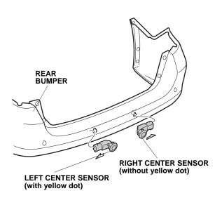
57. From the inside of the rear bumper, insert the right center sensor clip (black) and left center sensor clip (white) to the right center sensor and left center sensor.
