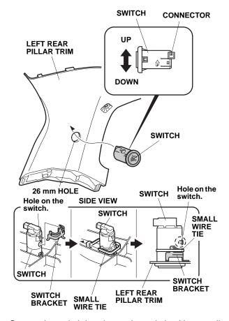
49. Secure the switch bracket to the switch with a small wire tie.
