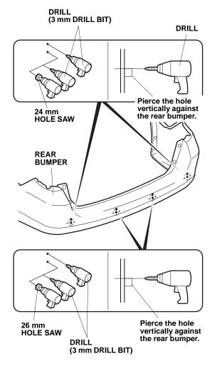
55. While wearing an eye protection, drill 3 mm hole at the four pierced marks on the center of the rear bumper from the outside. Widen the two lower holes with 26 mm hole saw as shown. Remove any burrs.
