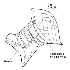
47. On the inside of the left rear pillar trim, measure from the inside of the ribs, and mark the pillar trim at the measurements shown. While wearing eye protection, drill a 3 mm hole at the marked position. Then drill with a 26 mm hole saw.
