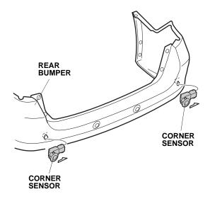
59. From the inside of the rear bumper, insert the two corner sensor clips to the two corner sensors.
