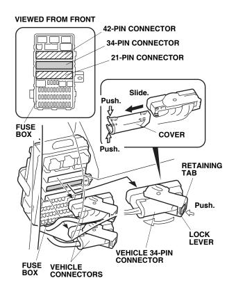
38. Get the fog light switch harness, and insert the white and pink switch harness terminals into the appropriate cavities of the white vehicle 34-pin connector.
