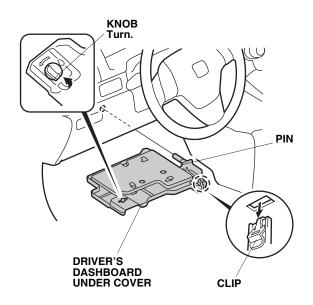
27. Remove the driver's dashboard lower cover (seven clips and two hooks).
