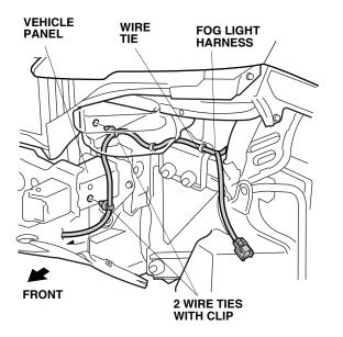
20. Route the fog light harness under the bumper beam towards the right side of the vehicle. Secure the fog light harness.
