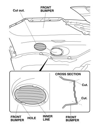
8. Cut off the four ribs on the front bumper as shown. Remove any burrs. Remove the masking tape.
