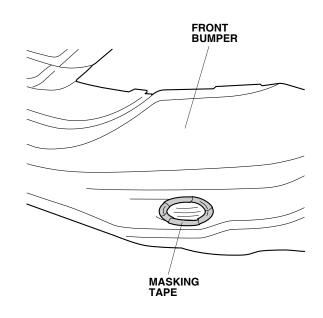
7. Using a utility knife, cut along the inner line of the hole as shown. Take care not to damage the front bumper.
