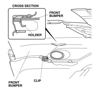
Install the left fog light to the front bumper using three 5 x 14 mm self-tapping screws.
