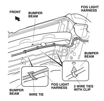
21. Using isopropyl alcohol on a shop towel, clean the bumper beam surface where the harness tape will attach.
