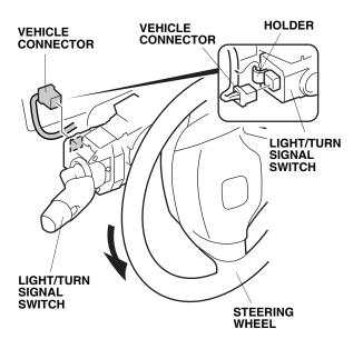
43. Remove the two self-tapping screws from the light/ turn signal switch. While pushing the retaining tab, slide the light/turn signal switch, and remove it from the steering column. While removing, do not hold the light/turn signal switch by the lever.
