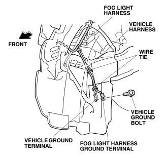
16. Secure the fog light harness to the vehicle harness with two wire ties.
