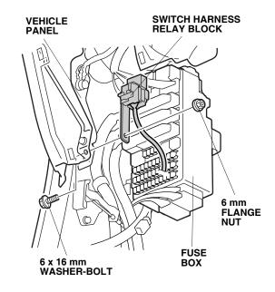
36. Plug the switch harness 2-pin connector into the vehicle harness 2-pin connector. Secure the switch harness to the vehicle harness using two wire ties.
