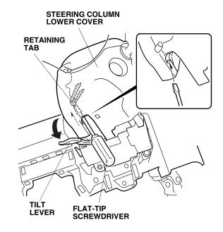
31. Remove the steering column upper cover (two retaining tabs on each side).
