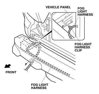
24. Secure four remaining fog light harness clips to the holes in the vehicle panel.
