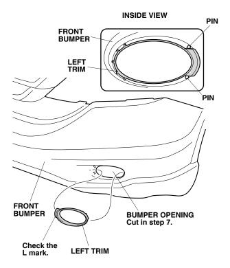
10. Inside the bumper, install one clip to the front bumper.
