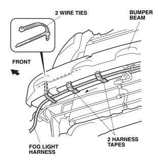
22. Continue routing the fog light harness along the bumper beam to the right side of the vehicle. Secure the fog light harness under the bumper beam using two adhesive tapes and two wire ties connected together.
