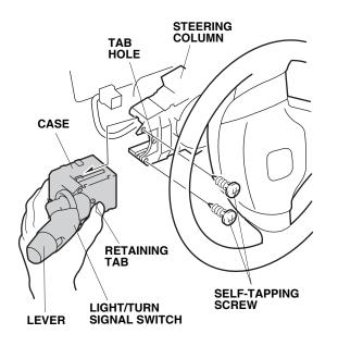
44. Install the new light/turn signal switch on the steering column with two self-tapping screws. While installing do not hold the light switch by the lever.
