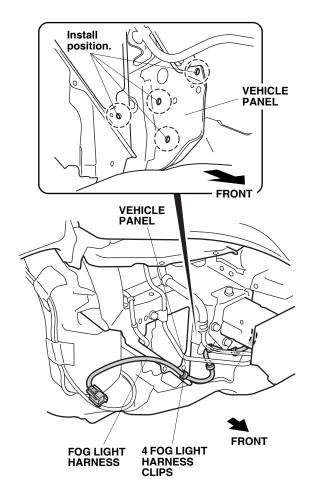
25. Reinstall the inner fender. With the help of an assistant, bring the front bumper close to the vehicle, and plug the fog light harness 2-pin connectors into the right and left fog lights. Reinstall the front bumper.
