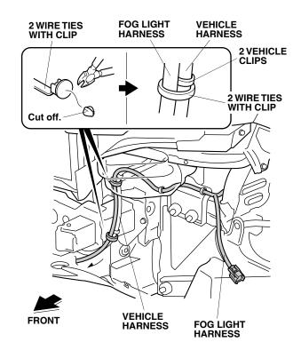
Without a Vehicle Harness: Secure the fog light harness to the bumper beam using two wire ties with clip and one wire tie.
