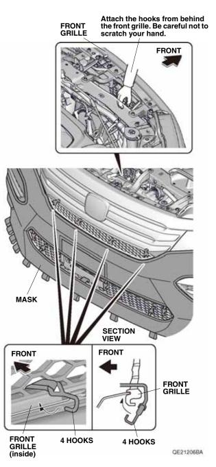
15. Attach five hooks to the inside edge of the front lower grille.
