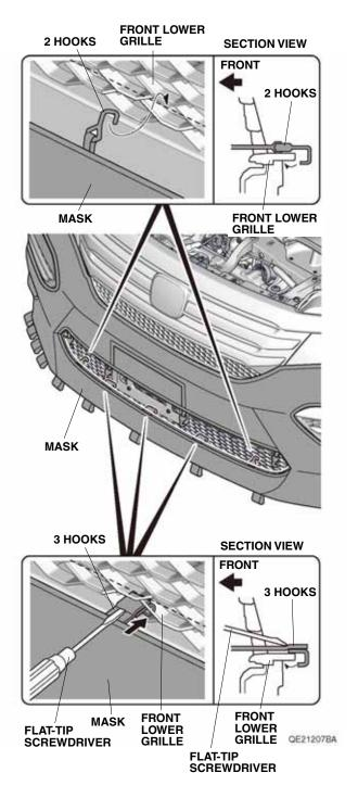
16. Attach four hooks to the inside edge of the front lower grille.
