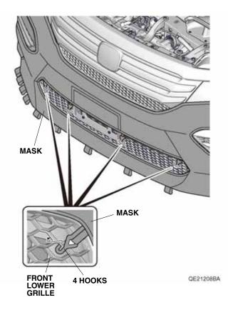
17. Route the elastic cord through the thirteen loops on the bottom of the mask. Attach one hook to the gap of the inner fender and front bumper. Stretch out the elastic cord after routing it through each loop then secure the other hook to the gap of the inner fender and front bumper on the other side.
