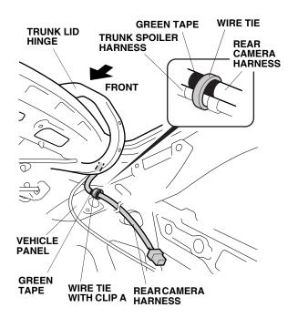
42. Route the rear camera harness towards the rear of the vehicle, and secure it to the vehicle panel hole with one wire tie with clip A. NOTE: If a trunk spoiler is installed, secure the rear camera harness to the trunk spoiler harness with one wire tie.
