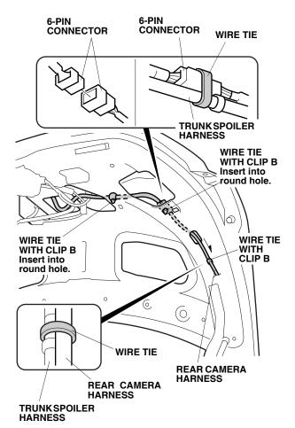
36. Secure the rear camera cord and the rear camera harness to the vehicle panel with three wire ties with clip B.
