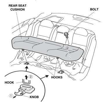
10. Remove the right seat side bolster (one bolt and release the one hook).
