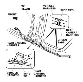
47. Route the rear camera harness through the passenger's door opening, and secure it to the vehicle harness with five wire ties.
