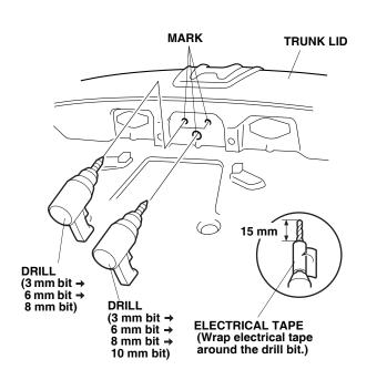
27. Install two well-nuts into the 8 mm holes.
