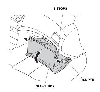
5. Remove the glove box (two screws).
