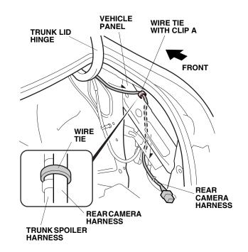
43. Route the rear camera harness along the vehicle harness, and secure it to the vehicle harness with six wire ties.
