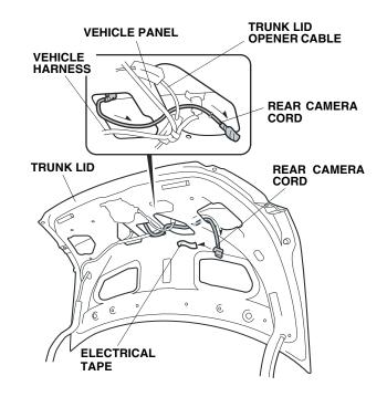
34. Remove the terminal lock from the 6-pin connector. Insert the rear camera terminals into the 6-pin connector. Verify each terminal position, and then reinstall the terminal lock.
