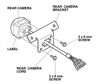
29. Wrap the terminals of the rear camera cord with electrical tape.
