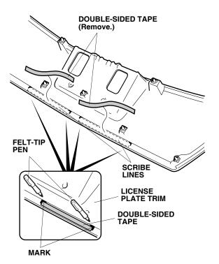
60. Remove the double-sided tape from the license plate trim. (Use 3M General Purpose Adhesive Cleaner, 3M #08984.)
