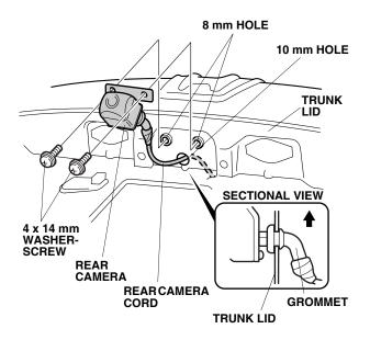
32. Install the rear camera assembly to the trunk lid using the two 4 x 14 mm washer-screws.
