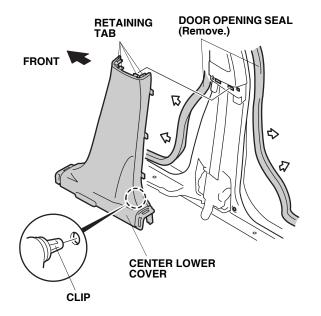
13. Remove the right center lower cover (one clip and four retaining tabs).
