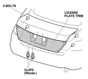
20. Insert the KTC trim tool (AP201-W) between the license plate trim and the trunk lid. Move the tool left and right to peel off the double-sided tape in between.
