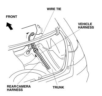
45. Route the rear camera harness forward along the vehicle harness, and secure it to the vehicle harness with four wire ties.
