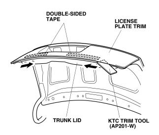
21. Pull out on the license plate trim and disengage the lower three clips. Do not remove the license plate trim yet.
