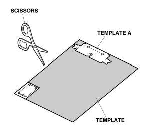
25. Tape template A on the trunk lid as shown. Lightly center punch the trunk lid at each of the three marks indicated on template A. Remove template A.
