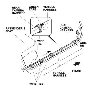
48. Route the rear camera harness up through the glove box opening, and secure it to the vehicle harness with five wire ties.
