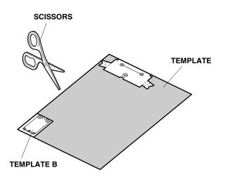
52. Attach template B to the license plate trim using tape.
