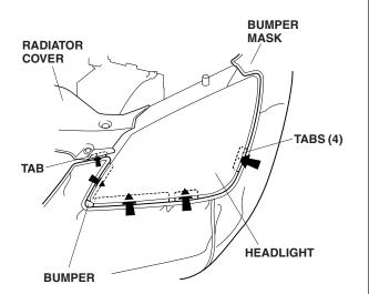
9. Insert the six tabs between the grille and the bumper.
