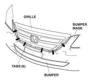
10. Attach the four elastic straps to the inside top edge of the bumper opening, and attach the six plastic hooks to the bottom inside edge of the bumper opening.
