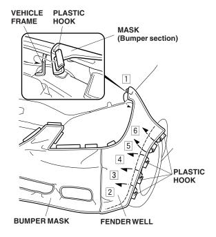
7. On both sides of the vehicle, attach the five plastic hooks between the fenderwell and the fender in the sequence shown.
