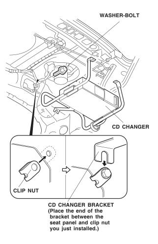
35. Loosely install the washer-bolt to the rear seat panel first. Then, place the end of the CD changer bracket between the seat panel and clip nut you just installed.
