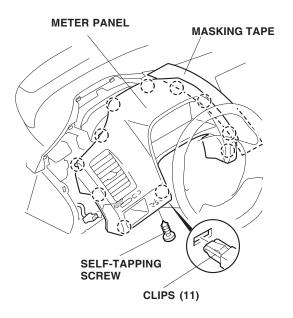
Apply masking tape to the instrument panel as shown, and remove the center panel (two bolts, ten retaining clips, and unplug the vehicle connectors).
