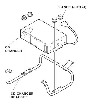
33. Wrap one EPT sealer around the BUS cable connector from the CD changer, then secure the BUS cable and connector to the CD changer bracket with two wire ties.
