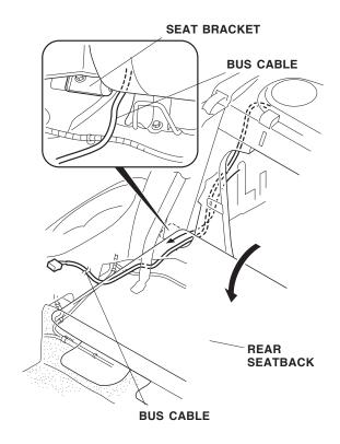
20. Lift up and lock the right rear seatback, then remove the clip that secures the floor carpet. Pull back the floor carpet
