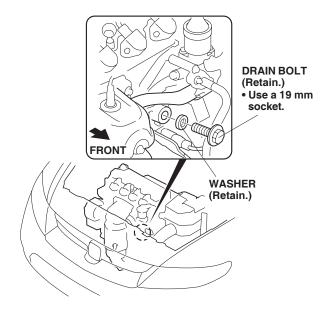
7. Install the new aluminum washer and the engine block heater into the bolt hole using a 24 mm socket and a torque wrench. Torque the engine block heater to 60 N·m (6 kgf·m, 44 lbf-ft).
