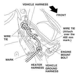
Route the heater harness to the back of the right headlight along the vehicle harness, then secure the harnesses with two wire ties in the areas shown.
