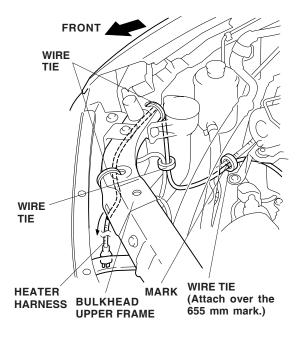
11. Route the heater harness to the side of the right headlight through the back of the bulkhead upper frame, then let it hang down toward the front. Secure the heater harness to the hole in the bulkhead upper frame with two wire ties in the areas shown.
