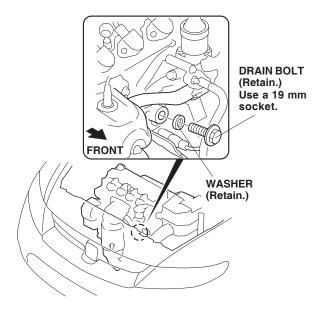
Install the new aluminum washer and the engine block heater into the bolt hole using a 24 mm socket and a torque wrench. Torque the engine block heater to 60 N·m (44 lb-ft).
