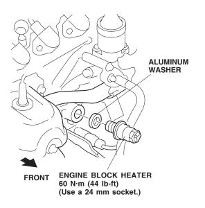
8. Plug the connector end of the heater harness into the engine block heater. Route the heater harness as shown and secure it to the vehicle bracket with one white wire tie at the white mark (point A) you made.
