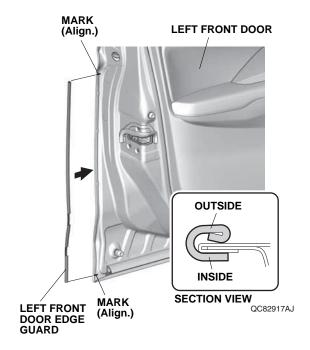
8. Starting at the feature line, use a rubber mallet to tap the left front door edge guard into position with a series of light taps, then work up and down. Once in place, do not attempt to remove, reposition, or reinstall the left front door edge guard.
