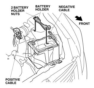
7. Remove the battery cover, battery, and battery box.
