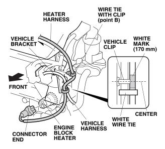
13. Route the heater harness as shown and secure the heater harness to the vehicle harness with one white wire tie at the 170 mm mark you made. Secure the one wire tie with clip (270 mm) to the vehicle bracket. 14. Route the heater harness as shown and secure it to the fan shroud rib with four black wire ties.
