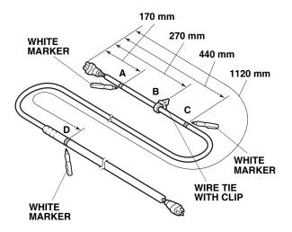
9. Using a white marker, mark the heater harness at the measurements shown.
