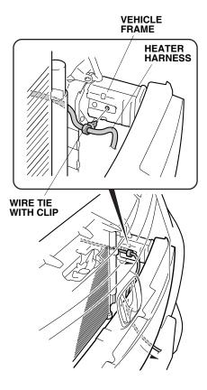
17. Route the heater harness inside the bumper and secure it with the three black wire ties.
