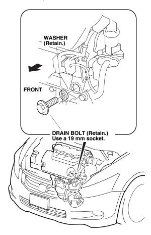
11. Install the engine block heater with the aluminum washer into the engine block using a 24 mm socket and a torque wrench. Torque the engine block heater to 60 N·m (44 lbf-ft).
