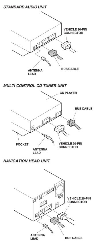
41. Connect the four vehicle connectors to the center panel, and reinstall the center panel.
