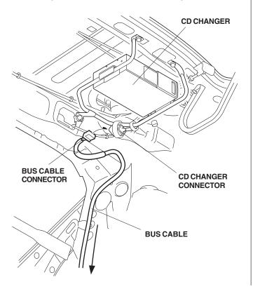
39. Fold the excess bus cable and secure the bus cable to the holes of the rear seat panel with the two wire ties with clip.
