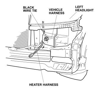
18. Route the heater harness as shown, and secure it to the vehicle harness with one black wire tie (point F).
