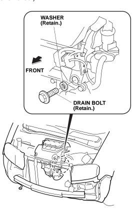
10. Install the engine block heater with aluminum washer into the engine block using a 24 mm socket and a torque wrench. Torque the engine block heater to 60 N·m ( 44 lbf·ft).
