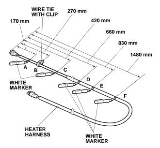
8. Using a white marker, mark the heater harness five times, using the measurements shown.
