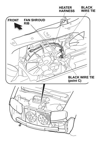
14. Secure the heater harness to the fan shroud rib with one black wire tie.
