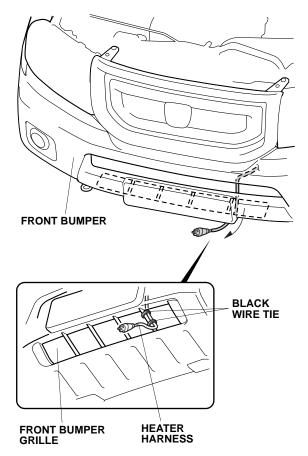
21. Route the heater harness as shown, and secure it to the front bumper grille with two black wire ties.
