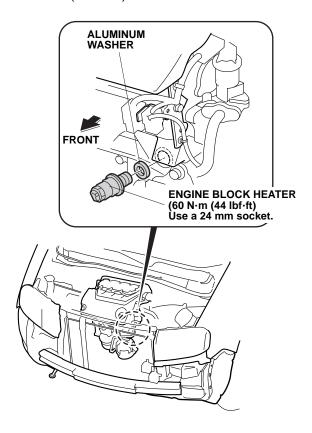
11. Plug the connector end of the heater harness into the engine block heater.
