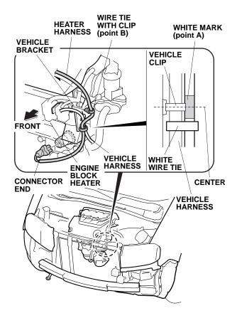
Route the heater harness as shown, and secure it to the vehicle harness with one white wire tie (point A). Secure the one wire tie with clip (point B) to the vehicle bracket. 13. Route the heater harness as shown, and secure it to the fan shroud rib with one black wire tie (point C).
