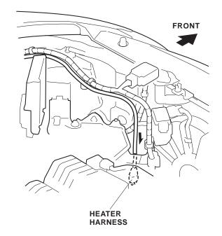
15. Secure the wire tie with clip that you installed on the heater harness at point B to the vehicle frame. Route the heater harness to the front bumper opening.
