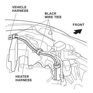
17. Route the heater harness on the inside of the bumper opening, and secure it to the grille with a black wire tie as shown.
