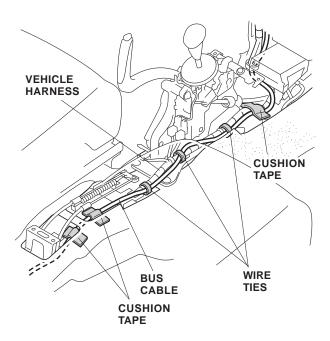
25. Using isopropyl alcohol on a shop towel, clean the areas where the cushion tapes will attach. Attach the bus cable to the floor panel with three cushion tapes in the areas shown.
