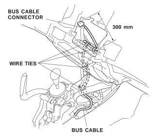
24. Along the center console area, secure the bus cable to the vehicle harness with three wire ties.
