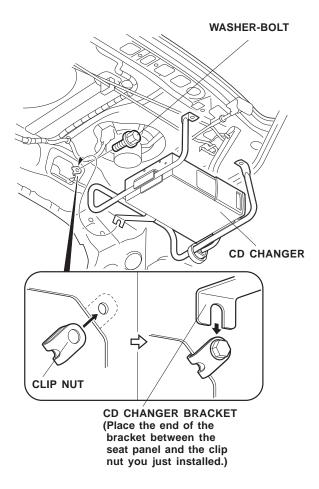
35. Loosely install the washer-bolt to the clip nut first. Place the end of the CD changer bracket between the seat panel and the clip nut you just installed.
