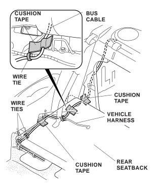
29. Attach the bus cable to the floor panel with the three cushion tapes in the areas shown.
