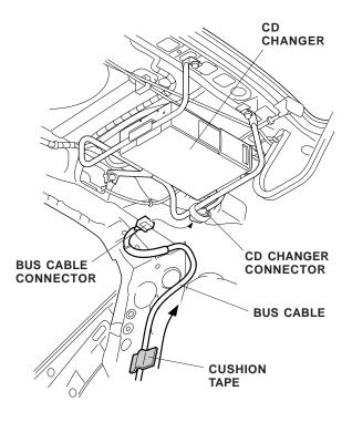
38. Fold the excess bus cable, and secure it to the holes in the rear seat panel with two wire ties with clips.
