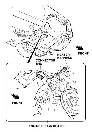
16. Route the heater harness along the engine block, and secure it to the engine block heater bracket with two wire ties with clip at point A and point B.
