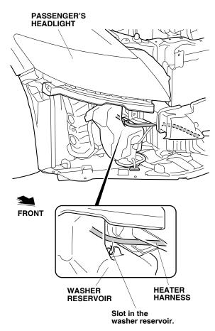
23. Align the white mark at point F to the vehicle clip on the front bumper beam cover, and secure the heater harness to the vehicle harness with one wire tie.
