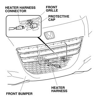
27. Attach the protective cap to the front grille, and plug the heater harness connector into the protective cap.
