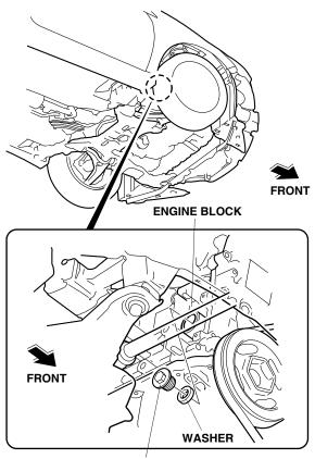
DRAIN BOLT Retain. Use a 19 mm socket. 11. Install the engine block heater with the aluminum washer into the bolt hole using a 24 mm socket and a torque wrench. Torque the engine block heater to 60 N·m (44 lbf·ft).
