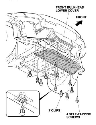
7. Remove the engine under cover (six self-tapping screws and four clips).
