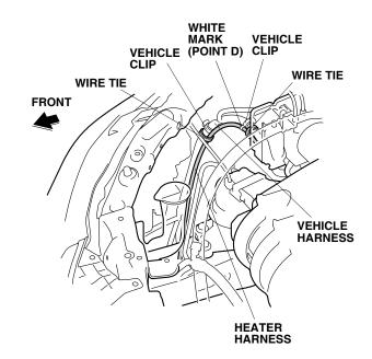
20. Route the heater harness forward, and secure it to the vehicle harness with one wire tie. Do not secure heater harness to the SRS harness.
