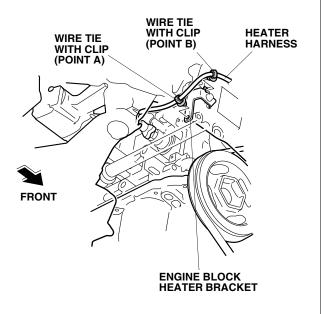
17. Route the heater harness through the engine compartment as shown.
