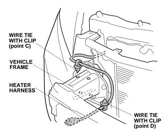
16. Bundle the excess of the heater harness. Using three black wire ties, secure the harness to the vehicle harness.
