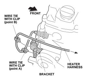
Route the heater harness as shown. Using two black wire ties, secure the heater harness to the vehicle harness.
