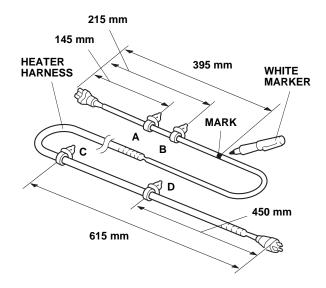
9. Plug the heater harness connector into the engine block heater. Temporarily place the entire heater harness on top of the engine.
