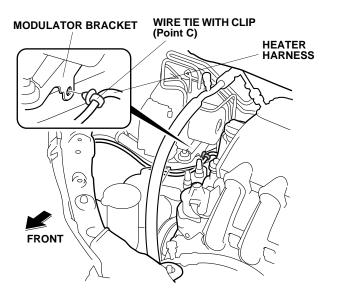
14. Route the heater harness along the vehicle harness and through the front bulkhead.
