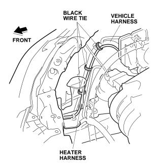
18. Route the heater harness under the frame, and secure it with one wire tie with clip (point E).
