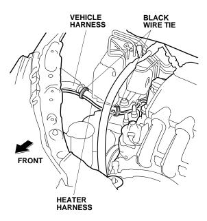
17. Secure the heater harness to the vehicle harness with three additional black wire ties.
