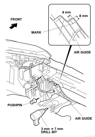
21. While wearing eye protection, drill the pierced mark to 7 mm. First drill with a 3 mm drill bit, and finish with a 7 mm drill.
