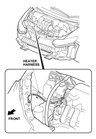
13. Secure the heater harness to the modulator bracket with one wire tie with clip (point C).
