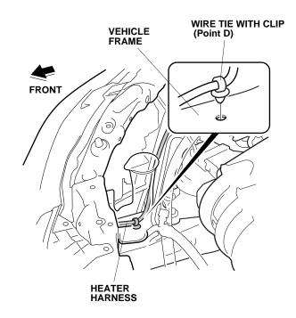
16. Secure the heater harness to the vehicle harness with two black wire ties.
