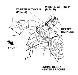
12. Route the heater harness through the engine compartment.
