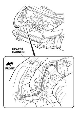
15. Secure the heater harness to the vehicle frame with one wire tie with clip (point D).
