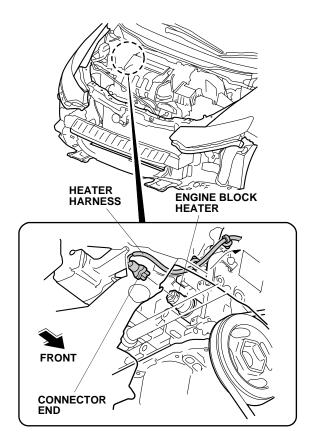
11. Route the heater harness up, and secure the two wire ties with clips (points A and B) to the bracket.
