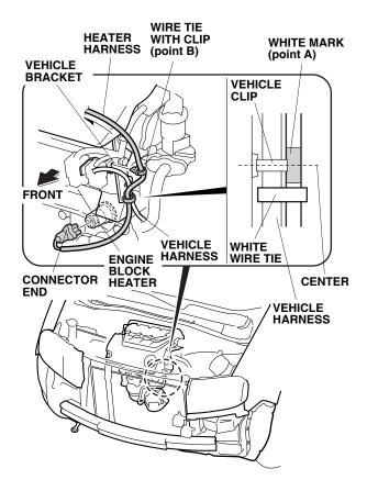
Route the heater harness as shown, and secure it to the vehicle harness with one white wire tie (point A). Secure the wire tie with clip (point B) to the vehicle bracket. 13. Route the heater harness as shown, and secure it to the fan shroud rib with one black wire tie (point C).
