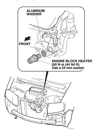
11. Plug the connector end of the heater harness into the engine block heater.
