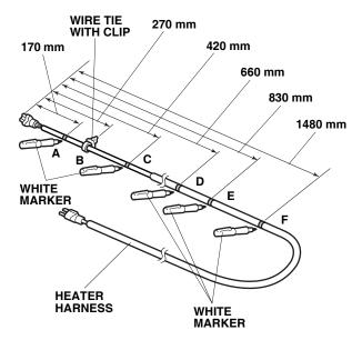
8. Using a white marker, mark the heater harness five times, using the measurements shown.
