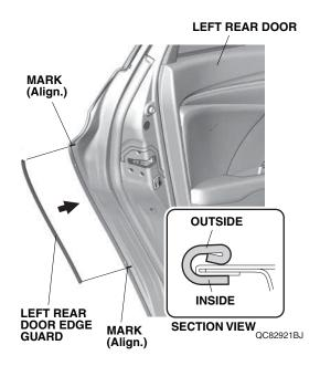
14. Starting at the upper side, use a rubber mallet to tap the left rear door edge guard into position with a series of light taps, then work down. Once in place, do not attempt to remove, reposition, or reinstall the left rear door edge guard.
