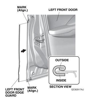
8. Starting at the feature line, use a rubber mallet to tap the left front door edge guard into position with a series of light taps, then work up and down. Once in place, do not attempt to remove, reposition, or reinstall the left front door edge guard.
