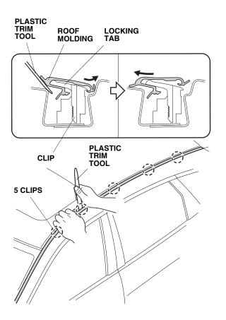
3. Pull the roof molding toward the outside of the vehicle to release the locking tabs, press the locking tabs towards the inside of the vehicle, and remove the roof molding from the vehicle. When removing the roof molding, start from the rear of vehicle and work toward the front.
