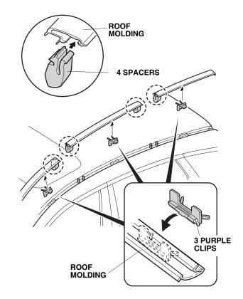
15. Reinstall the cut pieces of roof molding to the vehicle.
