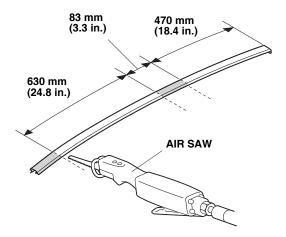
11. While wearing eye protection, use an air saw to cut the roof molding at each mark. Perform this step on a work bench.
