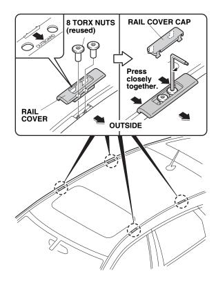
26. Snap the rail cover cap onto the rail cover. Pull the rail cover outward, and align the cover with the roof molding.
