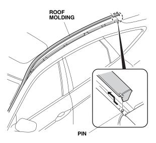
5. Tie a shop towel around the rear edge of the roof molding to avoid scratching the roof.
