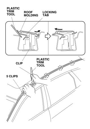
3. Pull the roof molding toward the outside of the vehicle to release the locking tabs, press the locking tabs towards the inside of the vehicle, and remove the roof molding from the vehicle. When removing the roof molding, start from the rear of vehicle and work toward the front. 4. Release the pin.
