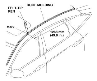
2. Using a plastic trim tool, pry up the edge of the roof molding in the areas shown.
