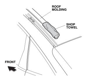
6. Place a blanket over the roof of the vehicle under the mark on the roof molding.
