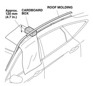
8. While wearing eye protection, use an air saw to cut the roof molding at the mark. Do not use a cutting wheel or shears to cut the roof molding, it will damage the roof molding. Have an assistant hold the rear edge near the shop towel while cutting.
